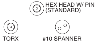
TAMPER RESISTANT SCREW HEADS OPTION SUFFIX- T3
